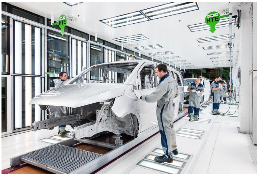
Figure 1. Check-men working on a production line, inspecting car body parts following the painting stage (image courtesy of Mercedes Benz España S.A.U., Vitoria Plant).
